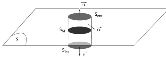
$$\phi_{\Sigma}(\vec{E}) = \iint_{\Sigma} \vec{E} \cdot d\vec{S} = \iint_{S_L} \vec{E} \cdot d\vec{S} + \iint_{S_{int}} \vec{E} \cdot d\vec{S} + \iint_{S_{ext}} \vec{E} \cdot d\vec{S} = E \cdot S_{ext} = \frac{\sigma \cdot S_M}{\epsilon_0}$$
