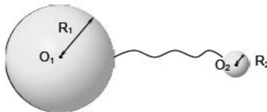
$$V(O_1) = V_1 = \frac{1}{4\pi\epsilon_0} \iint_{S_1} \frac{\sigma_1 dS}{R_1} \quad \left| \quad V(O_2) = V_2 = \frac{1}{4\pi\epsilon_0} \iint_{S_2} \frac{\sigma_2 dS}{R_2} \right.$$
